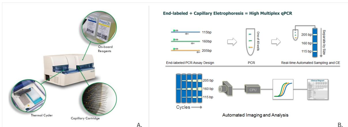
**Figure 2.** ICEPlex Technology. **A.** Components of the ICEPlex System. **B.** Principles of the multiplex real-time PCR detection.
