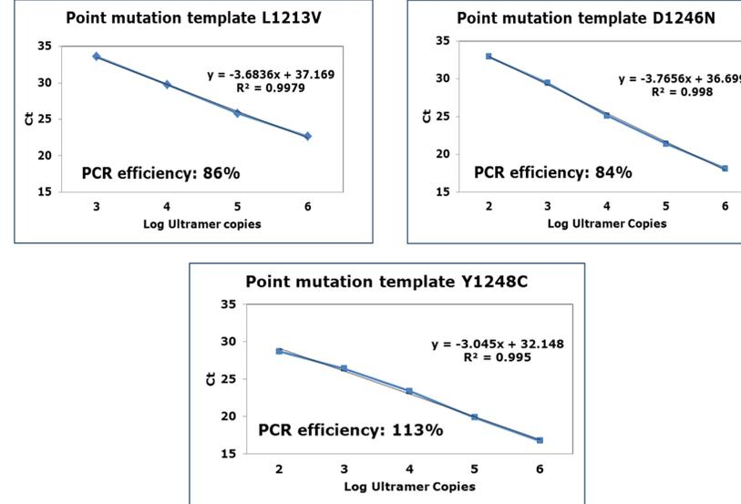
Fig 4. Serial dilutions of synthetic templates were tested to demonstrate the dynamic range of the assay and to calculate the PCR efficiency. ICEPlex cMET SNP Panel showed a dynamic range of 3-5 logs, and with PCR efficiency ranging from 80% to 120%.
