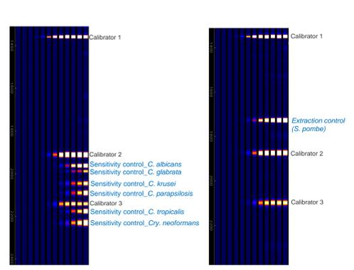
The ICEPlex Fungal Assay contains a sensitivity control (positive control for the presence of primers in the PCR reaction), an extraction control (*S. pombe*), and an optional Internal Control (data not shown here). The sensitivity control can be used either alone or in each PCR reaction.
