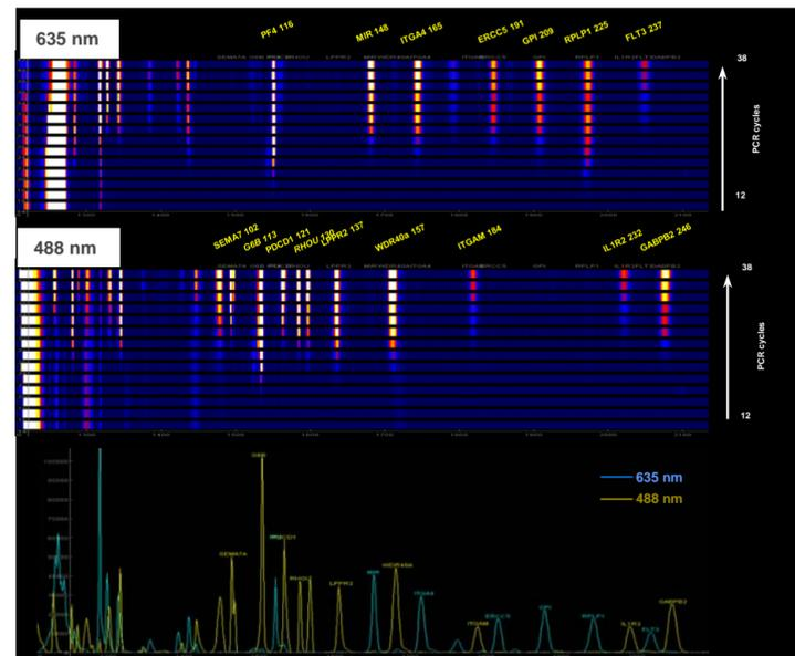
Top: Digital images from a single capillary showing the accumulation of PCR product over multiple cycles. Signal detected in 635nm and 488nm color channels. Note appearance and growth of signal from individual targets through amplification course.
