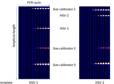
Figure 4. High specificity in detection of HSV-1 and -2 in a single PCR reaction.
